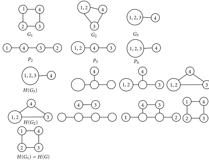
FIGURE 1: Example of a cactus construction for a 4-node ring topology. The top “row” gives the graphs  $G_i$ , for  $i = 1, \dots, r$ . The second row gives the paths  $P_i$ , for  $i = 2, \dots, N$ . The third row presents the first iteration of the for loop in algorithm Build-Cactus, while the fourth row presents the last iteration. The last row presents the cactus representation of the ring, which is a ring itself.
