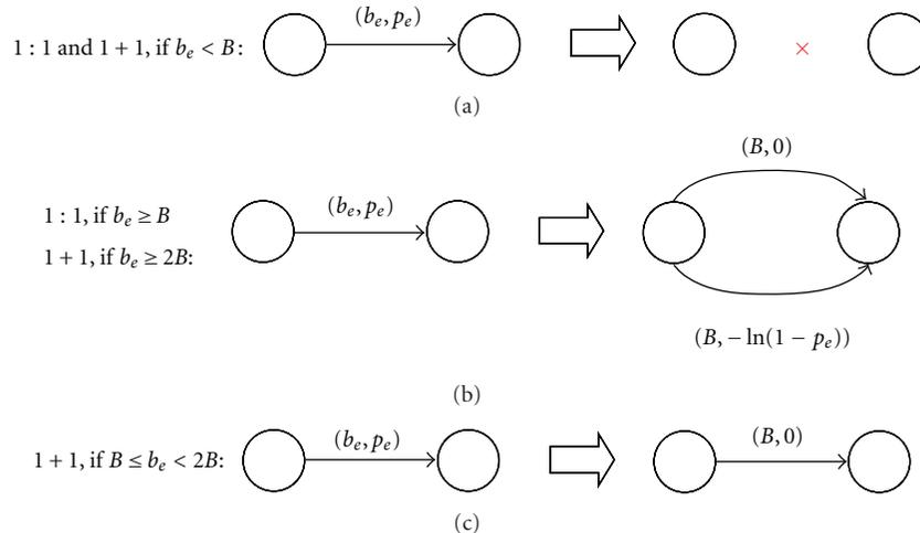
FIGURE 2: Graph transformation for the  $p$ -survivable- $B$ -bandwidth problem. For each link  $e$  with capacity  $b_e$  and failure probability  $p_e$ , the new links consist of a bandwidth-weight pair.
